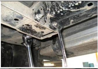
8. Before fitting transmission panel the mounting bracket needs to be attached to the rear of cross member. As shown in photo remove mounting nuts from gearbox cross member. NOTE: If you have side rails fitted it may be required to orientate bolts so they are placed in from front to back.
