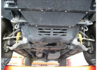
1. Remove O.E stone shields and retain mounting bolts for later use. If fitting an ARB recovery system do so now and refer step 2.
