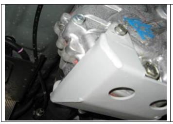
12. Remove original transfer case shield and retain bolts. Fit transfer panel as shown using original bolts. A drip tray will not be required for this procedure.
