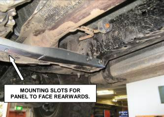
9. Mount and secure bracket to the 4 bolts on vehicle cross member. *Tighten cross member bolts to specified torque.*
