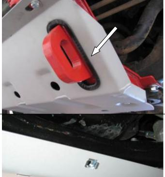
3. Fit rubber edging as shown before fitting panel to vehicle.
