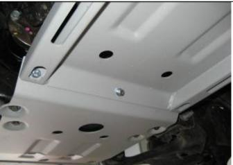
Lift transmission panel into place and secure to sump panel using 3 x M8 bolts, spring washers and flat washers supplied. Leave finger tight.
