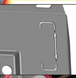
2. Using a marker pen and ruler joint the two 'U' shaped cut outs. Use masking tape to cover the outside edges of the drawn lines. Cut along lines using grinder with cutting disc to remove the rectangular section. De-burr and paint edges.
