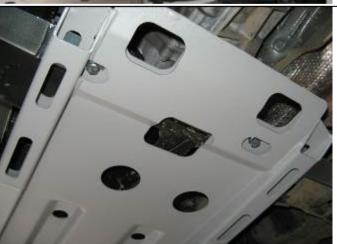
11. Secure panel to mounting bracket using 2 x M8 bolts, spring washers, flat washers AND flange nuts supplied. *When satisfied tighten all bolts to specified torque*.
